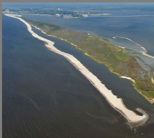
Thin layer sediment placement site at Deer Island Preserve to restore 100 acres of marsh habitat. Photo taken from the Engineering With Nature website (EWN 2024)
